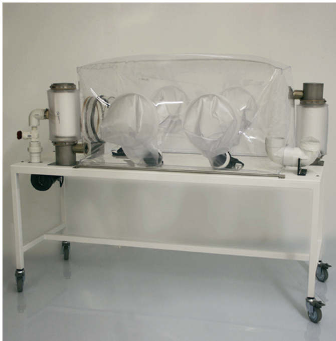
Pictured above is a 4' x 2' x 2' positive pressure, germ-free surgical isolator shown with the optional dip tube used for transferring items into the unit through an iodine bath.
